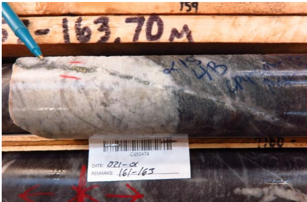
Photo 4. O21-01 at 159.8m – Epithermal style chalcopyrite-molybdenite-bornite veinlet cutting Microgranite and YTT (Orbit Zone).
