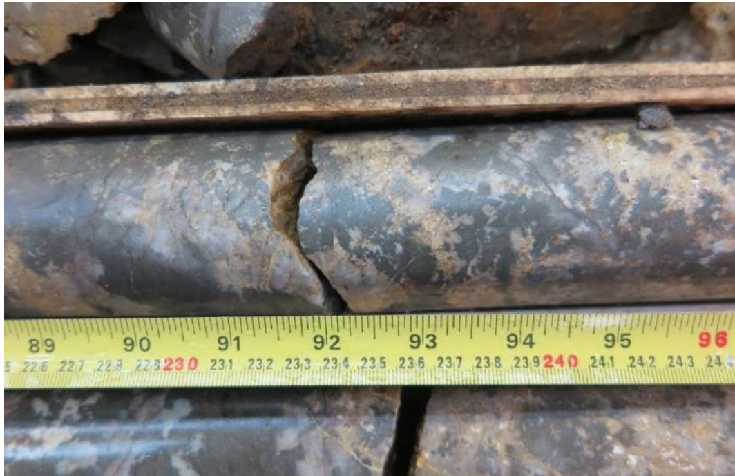
Photo 3. N21-05 at 174.14m – Semi-massive sulphide (marcasite +/- pyrite dominant) replacement within iron carbonate altered YTT (Big Creek South Fault area).
